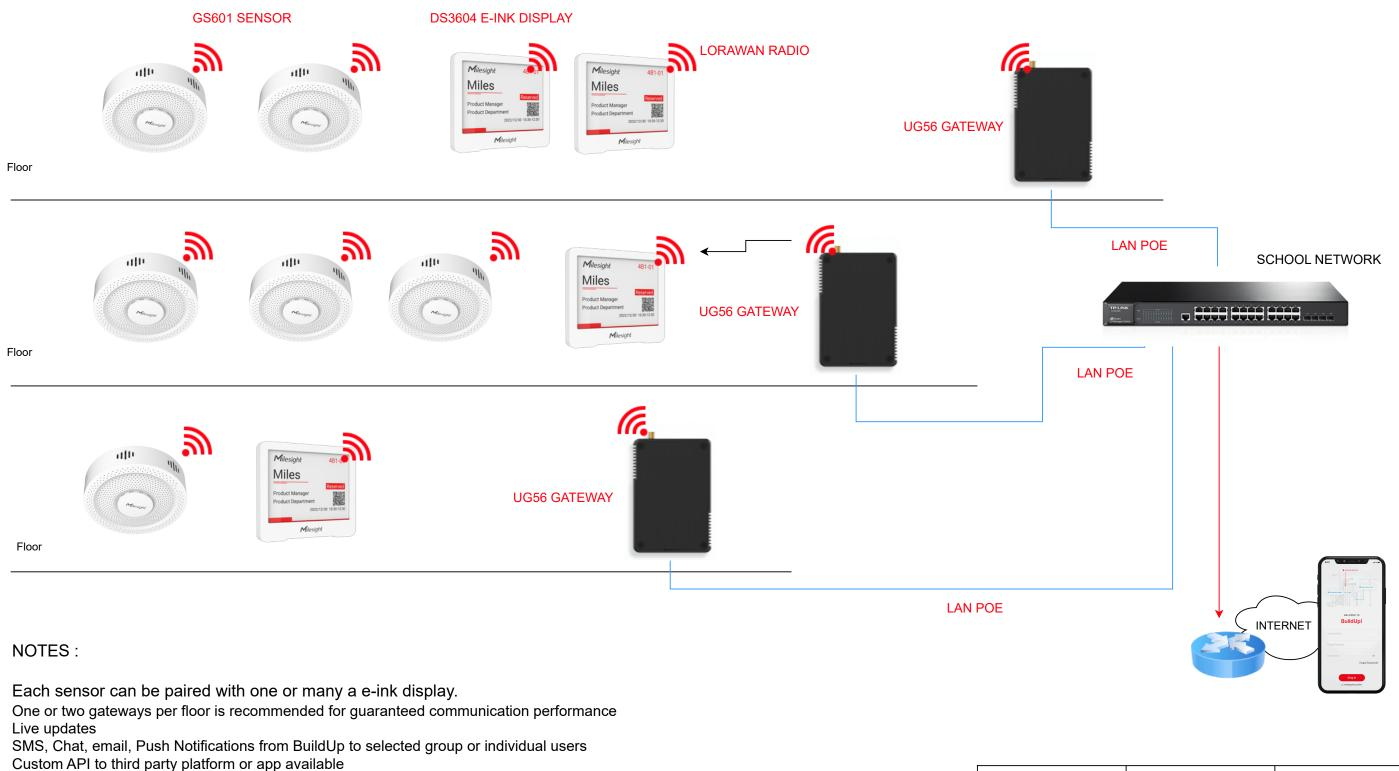
Sensors require 5VDC 1A with USB-C or PoE power
